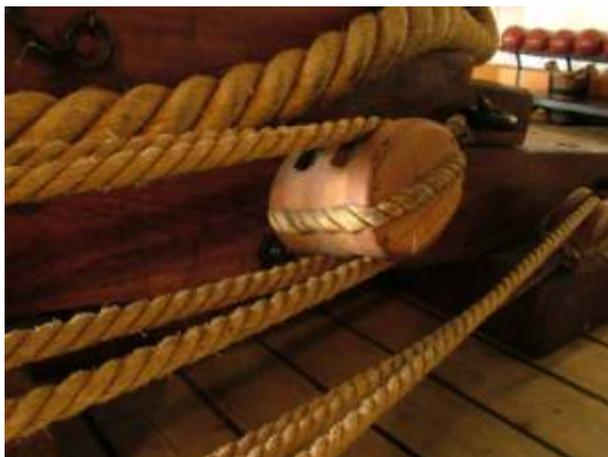
A pulley block used to move one of the *Warrior's* 68 pounder muzzle-loading guns
