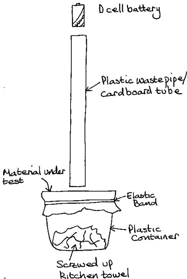
Start off by screwing up some kitchen towel and placing it in the bottom of the plastic container. This will cushion the fall of the battery and stop it from breaking open or damaging your container and the floor/table it might be resting on.
