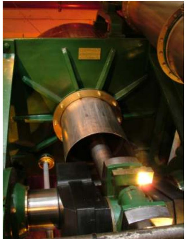
One of the twin pistons in *Warrior's* horizontal trunk engine
