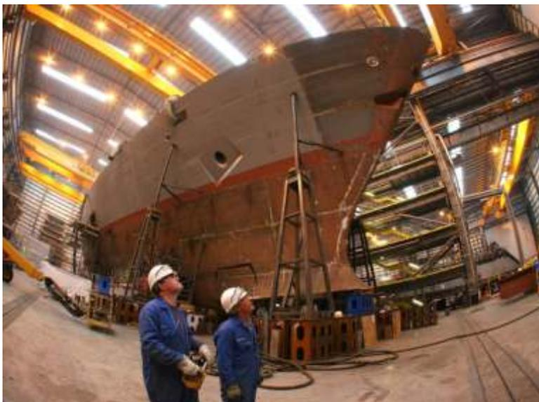
A Type 45 bow section under construction in the VT Ship Assembly Hall in Portsmouth
