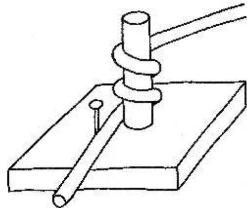
The coiling must be done carefully so that the copper tube does not collapse when bent.
